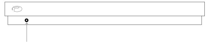
**Standby** – Toggles the player between normal operation and standby. In standby, the unit enters a low-power mode. The LED in the standby button is lit when in standby, and is off in normal operation (assuming the rear panel switch is turned on).
