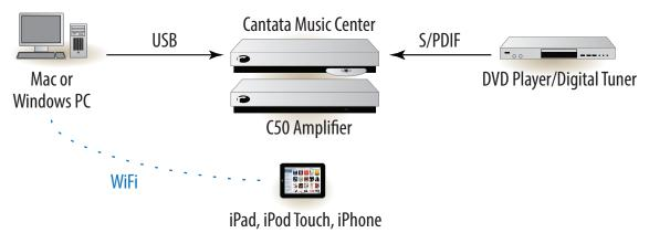
The Cantata Music Center serves as the "digital hub" of a high-end system featuring traditional S/PDIF inputs, an on-board CD transport, as well as playback over asynchronous USB from a computer.
